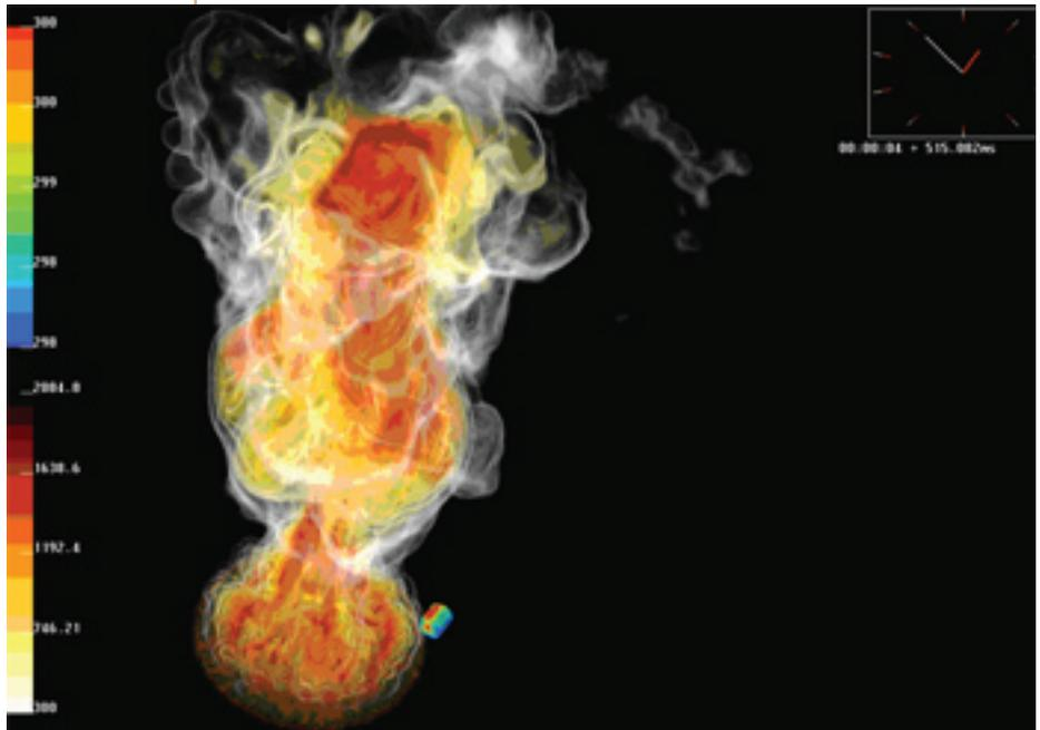
LES fire simulation showing volume rendered temperature and the resulting temperature of a nearby container.
